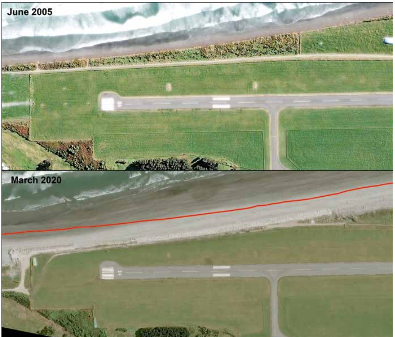
Photo: Very high resolution (30-50 cm) satellite imagery used to determine rates of shoreline change around NZ. Example shows 50 m of coastal erosion near Westport Airport between 2005 and 2020.
